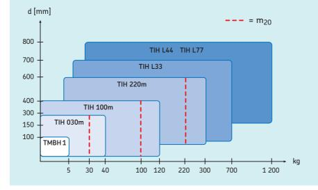
The comprehensive range of SKF induction heaters is suitable for most bearing heating applications. The chart gives general information on choosing an induction heater for bearing heating applications <sup>3</sup>).
