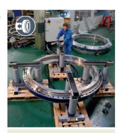
SKF can configure the type of TIH MC series heater required, depending on the application. For additional information, contact your SKF authorised distributor
