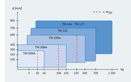
The comprehensive range of SKF induction heaters is suitable for most bearing heating applications. The chart gives general information on choosing an induction heater for bearing heating applications <sup>1)</sup>.
