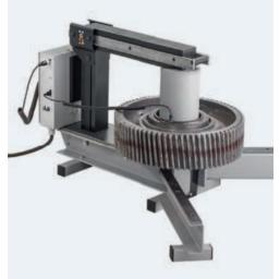
The TIH L MB heats non-bearing workpieces up to 600 kg (1 323 lb), depending on the model.
